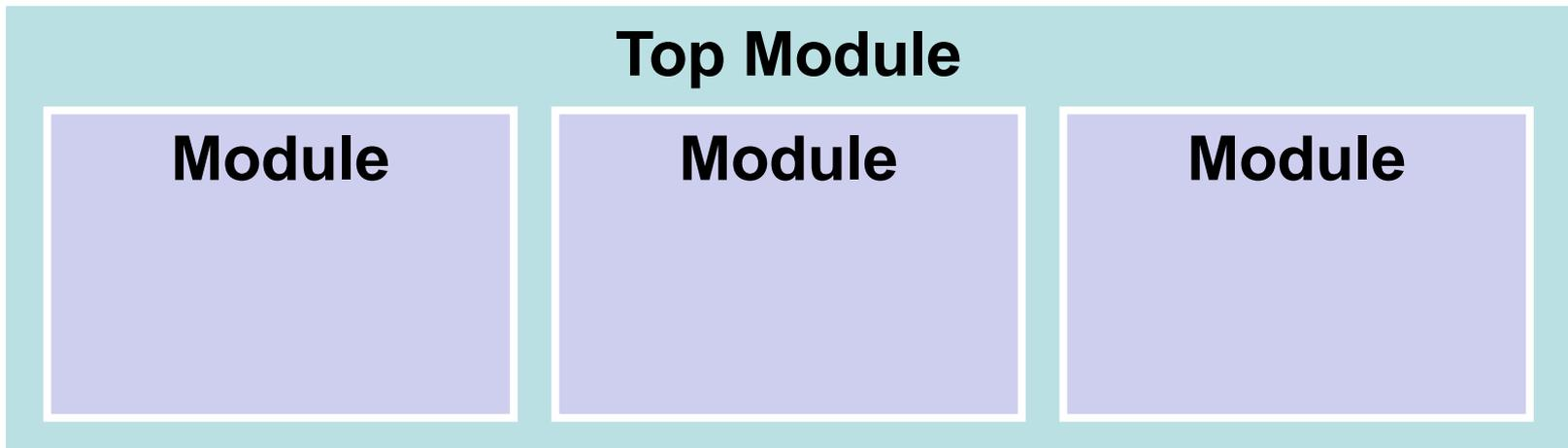
Connected by relating **I/O** and **internal** wires
